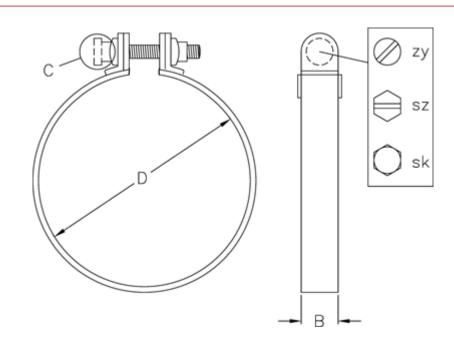
C (screw type) = SK Diameter D = 211 Width B = 25
